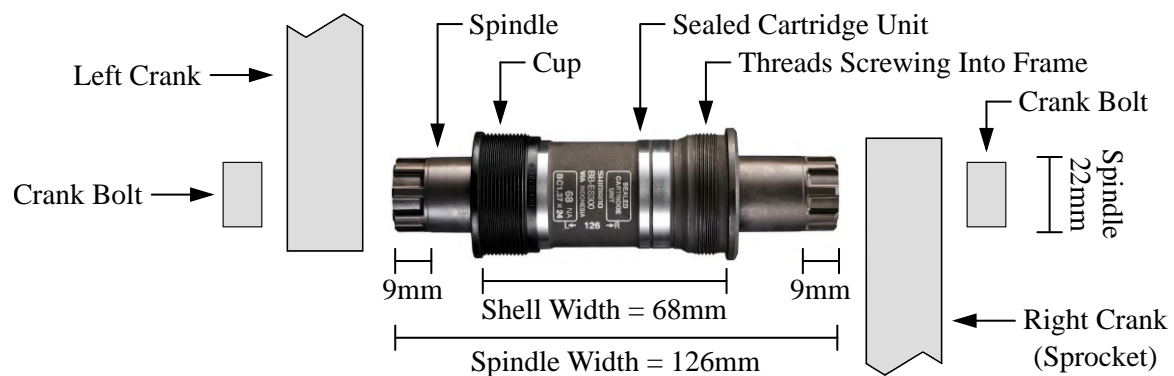
Figure 45: Example of the Shimano Octalink V2 BB-ES300 bottom bracket [105].
